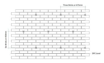
Diagram 1C - Typical drilling at roof or eaves level detail
