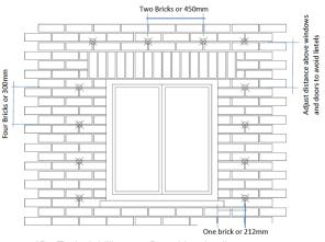
Diagram 1D - Typical drilling at a Party Line detail
